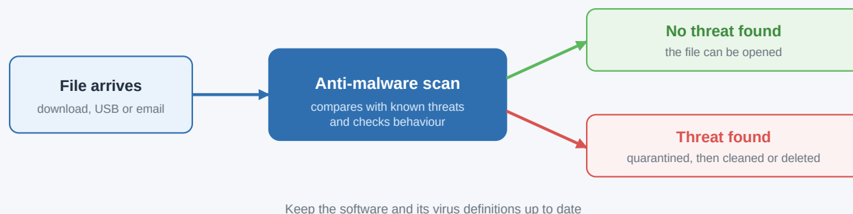
Figure 10: How anti-malware software checks a file
